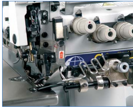
OV 614-240 PD-04 • 2 needle 4 thread double chainstitch with piping device
