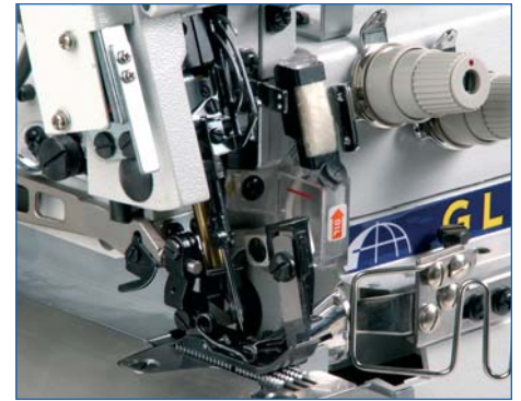
OV 614-408-TC • 2 needle 4 thread double chainstitch with Tape cutter
