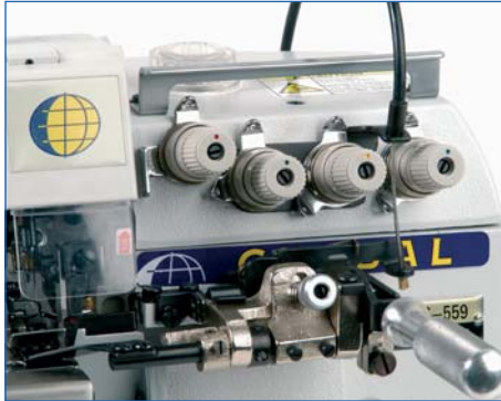
OV 616-559 - 5 thread with ruffling device
