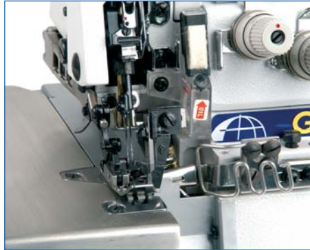
OV 616-330 BD-05 - 5 thread with binding device
